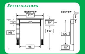
Generally designed to suit 8' wide x 10' high openings. The series D300 is used on higher door openings when a variety of trailer heights are being serviced.
